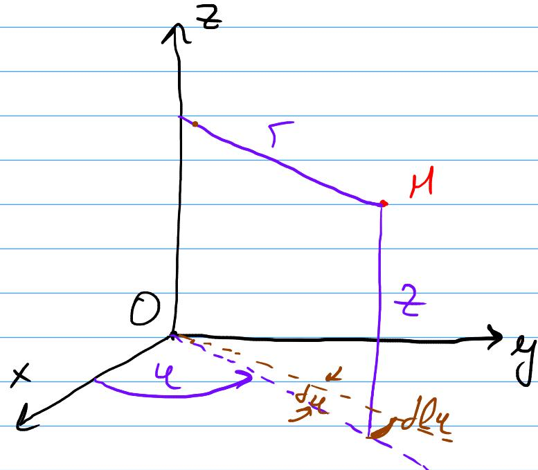
$$M(r, \varphi, z) \quad r \geq 0, -\pi < \varphi \leq \pi, -\infty < z < \infty$$
