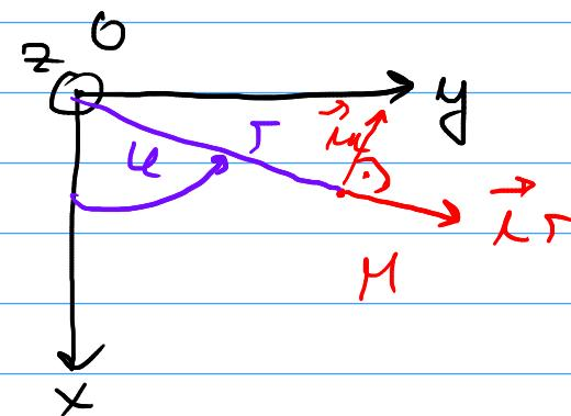
$$\begin{aligned}\vec{i}_r &= \cos \varphi \vec{i}_x + \sin \varphi \vec{i}_y \\ \vec{i}_\varphi &= -\sin \varphi \vec{i}_x + \cos \varphi \vec{i}_y \\ \vec{i}_z &\end{aligned}$$
