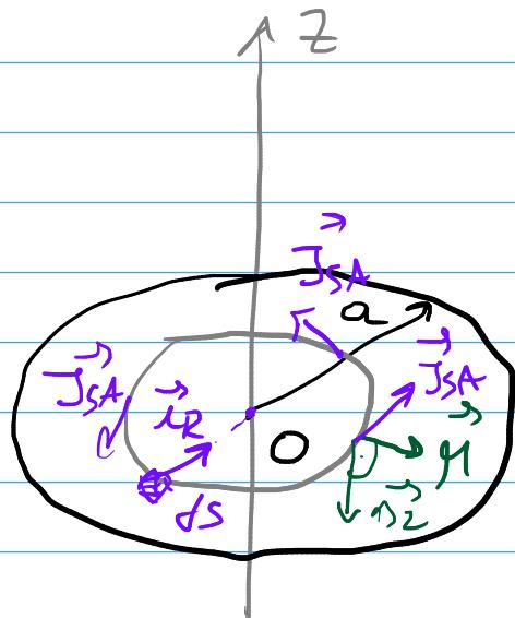
$$\vec{B} = \frac{\mu_0}{4\pi} \int_S \frac{\vec{J}_S dS \times \vec{\lambda}_R}{R^2}, \quad \vec{\lambda}_R = -\vec{\lambda}_r \quad \vec{\lambda}_r \times (-\vec{\lambda}_r) = \vec{\lambda}_z$$
